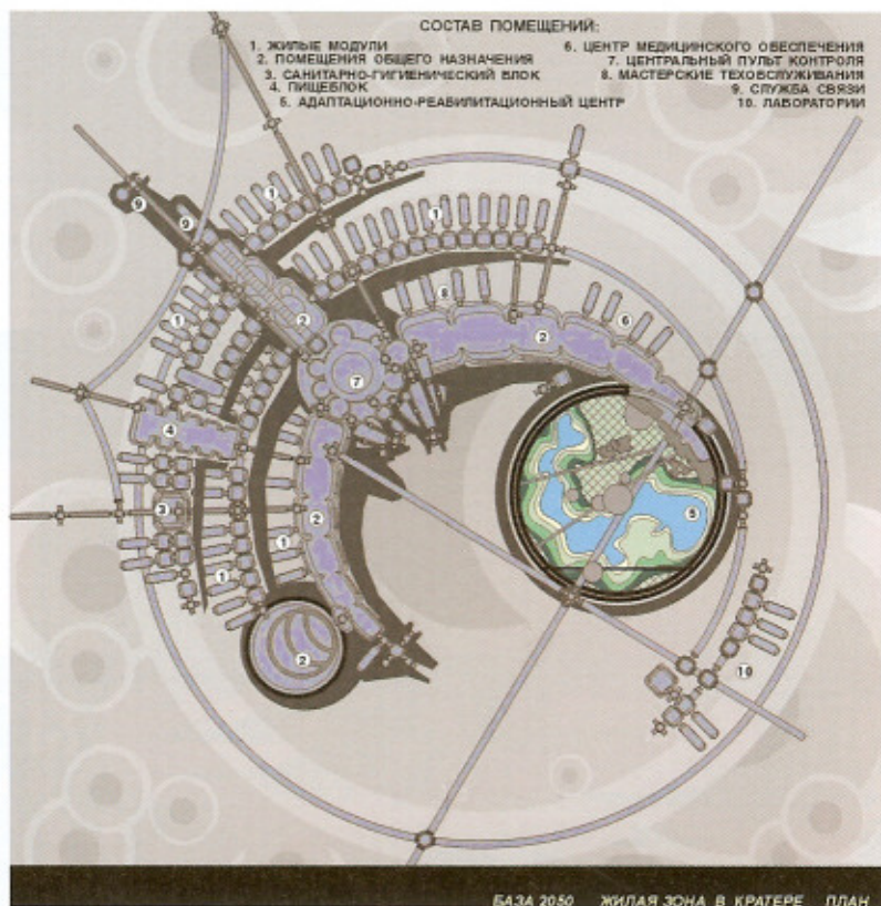
Plate 14 Manned base in crater: plan view. Legend: 1. inhabited modules 2. general purposes 3. clean facilities 4. kitchens 5. adaptation and rehabilitation 6. medical facilities 7. control center 8. maintenance 9. communications 10. labs. (Courtesy Vladislav Shevchenko) See Fig. 11.9 on page 354.
